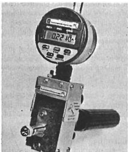
Gaging internal threads
